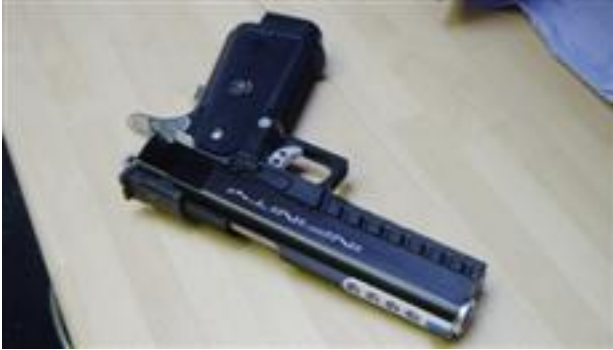
SVI Prokiller Mark 2 fitted with 10.5" barrel (F10) and PGC 1st generation F3.9 Metal slide with revised brass blowback chamber
