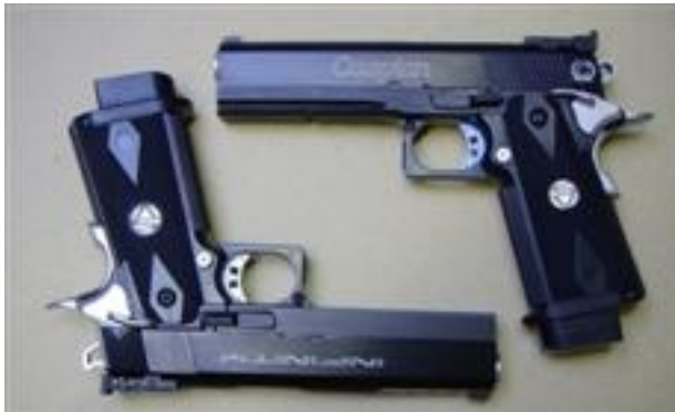
SVI pair - 5" Railed using SD Caspian slide and SVI Hybrid using custom milled SD 5" Infinity slide
